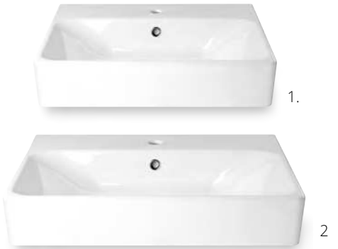
Quantum Square Slabtop Ceramic sit-on washbasins 1. w: 500mm d: 440mm h: 130mm 2. w: 600mm d: 440mm h: 130mm Available in two sizes, both featuring one tap hole and integral overflow for use with a slotted waste.
